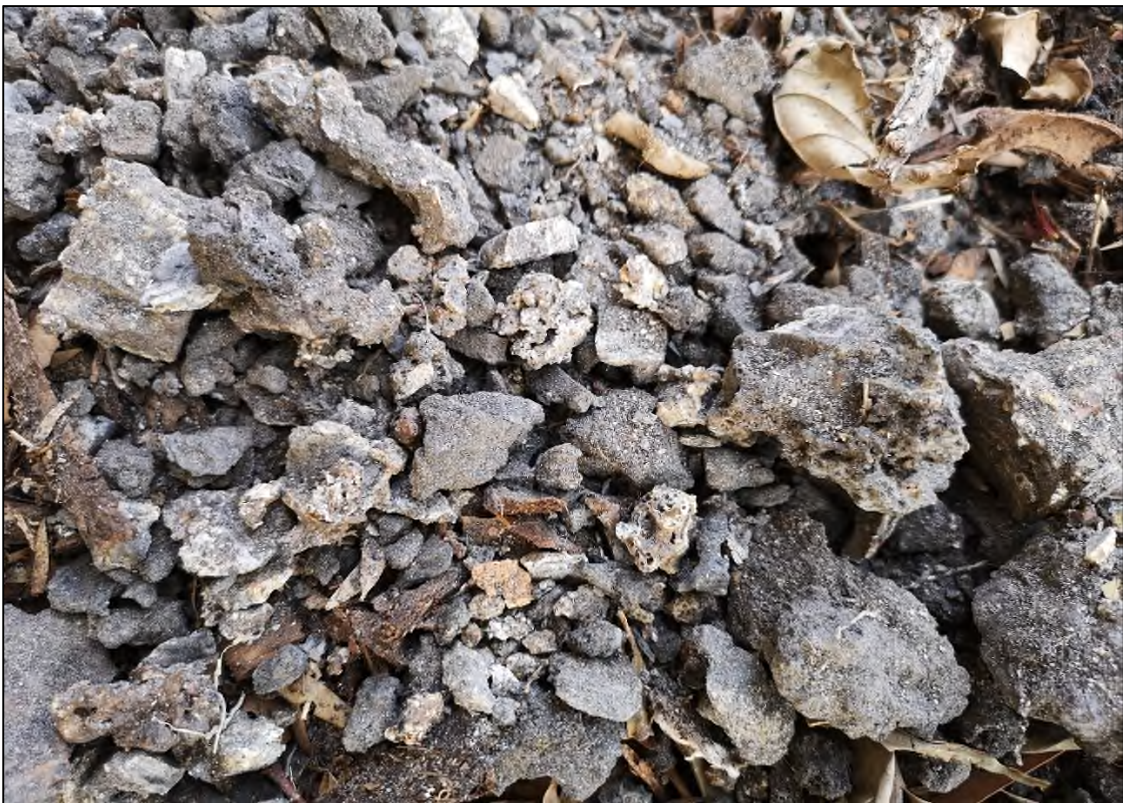
Photograph 6: Slag type material encountered in sample location along the external southern wall of the main hall building.
